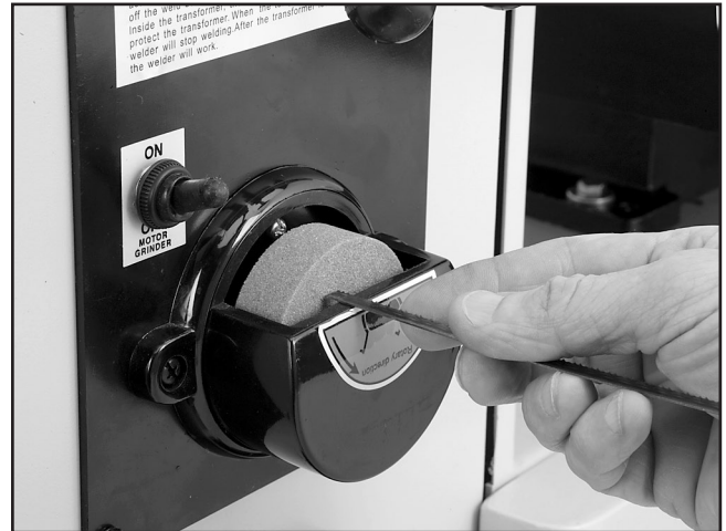
Figure 27. Using the grinder to square up the blade end.
